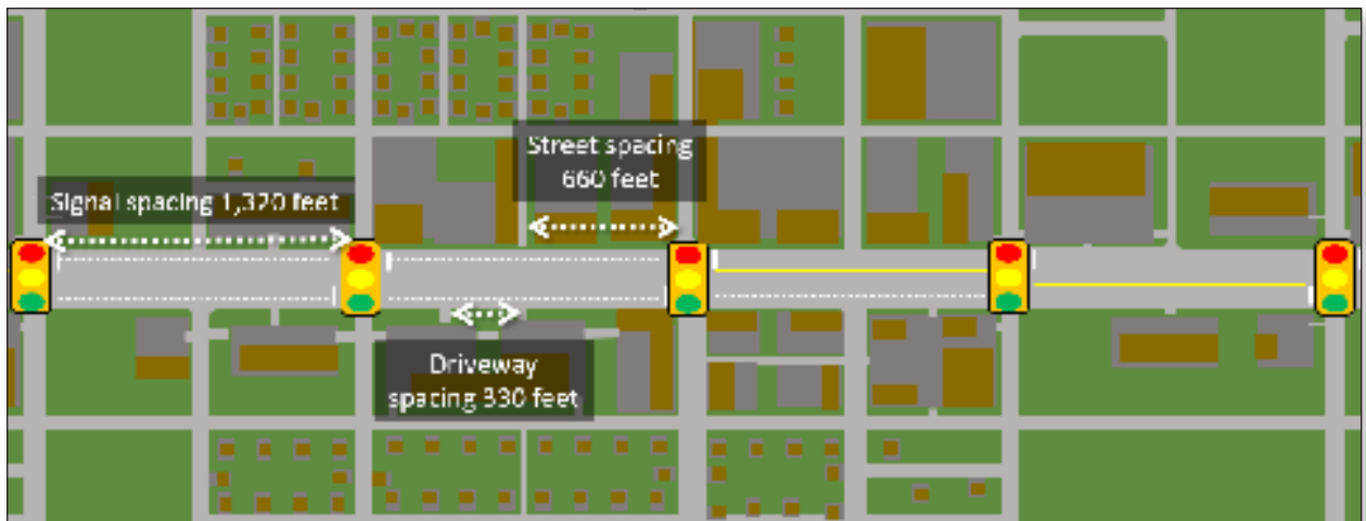
FIGURE 3-18. CLASS V DIAGRAM WITHOUT MEDIAN
