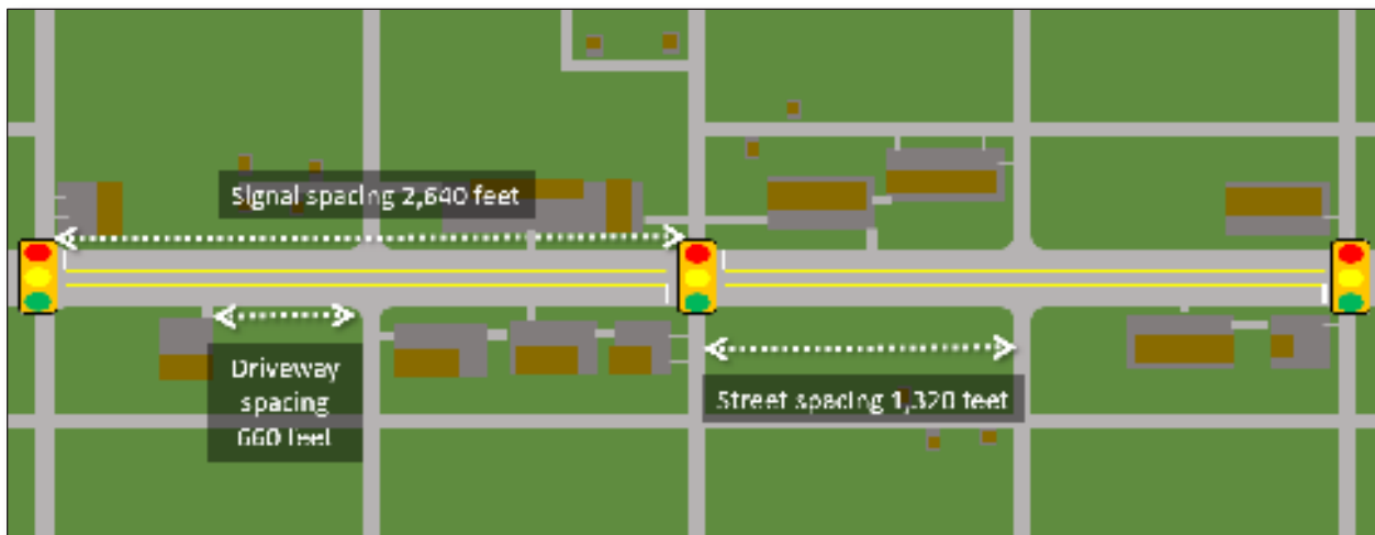
FIGURE 3-10. CLASS III DIAGRAM WITHOUT MEDIAN
