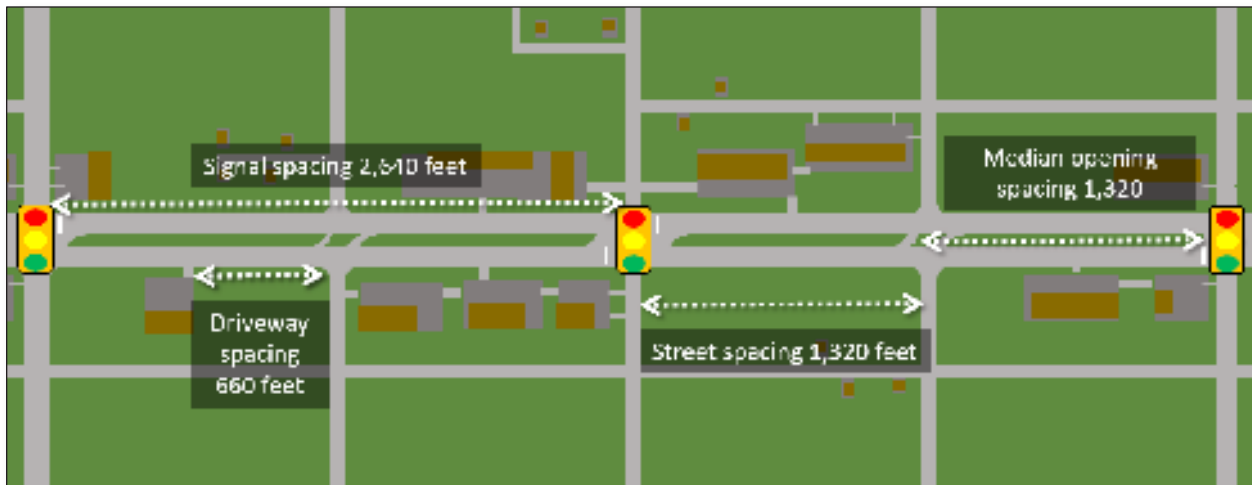
FIGURE 3-11. CLASS III DIAGRAM WITH MEDIAN
