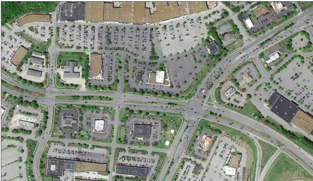
FIGURE 4-2. CROSS ACCESS AND REAR ACCESS ROADS
