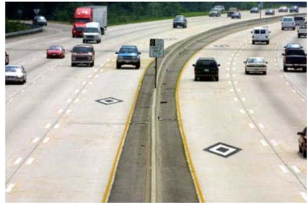
The need for weaving distance can often limit the number of access points that can be provided. On the other hand, lengthening each access point can sometimes allow closer spacing between access points, since drivers feel less rushed to make a weave maneuver. Taken to the extreme, access can be allowed for the entire length of the facility. Striping and signing are used to indicate that the driver is entering a managed lane. Enforcement on facilities of this type, particularly if it is a HOT lane rather than an express lane, can become problematic. Figure 9 — Double White Skip Access Point to HOV Lane in Virginia
